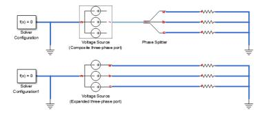
The top circuit uses a Voltage Source block with a composite three-phase port ~. The bottom circuit uses a Voltage Source block with expanded electrical conserving ports a, b, and c. In each circuit, the instantaneous phase voltages and currents are the same.
