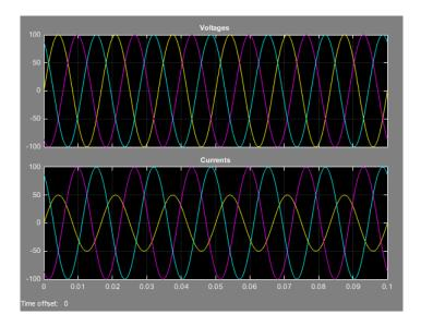
In this version of the model, one phase of the three-phase load has twice the resistance of the other two. Therefore, half as much current flows in that phase, as the second plot shows. However, because the load remains purely resistive, the voltage and current remain in phase with each other.
