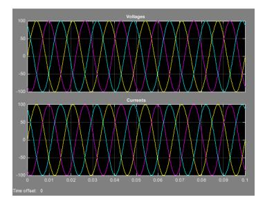
In this example, the **Component structure** parameter of the RLC block specifies that the electrical characteristics of the three-phase load are purely resistive. Therefore, for each phase of the three-phase system, the voltage and current remain in phase with each other. Because the resistance in each phase is  $\mathbf{1}\ \Omega$ , the magnitude of the phase voltage is equal to the magnitude of the phase current.
