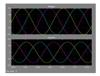
In "Build a Simple Three-Phase Model" on page 3-2, the electrical characteristics of three-phase load are purely resistive. In this model, the **Component structure** parameter of the RLC block is set to **Series** RL, meaning that the load has an inductive characteristic. The current flowing in each phase lags the voltage.
